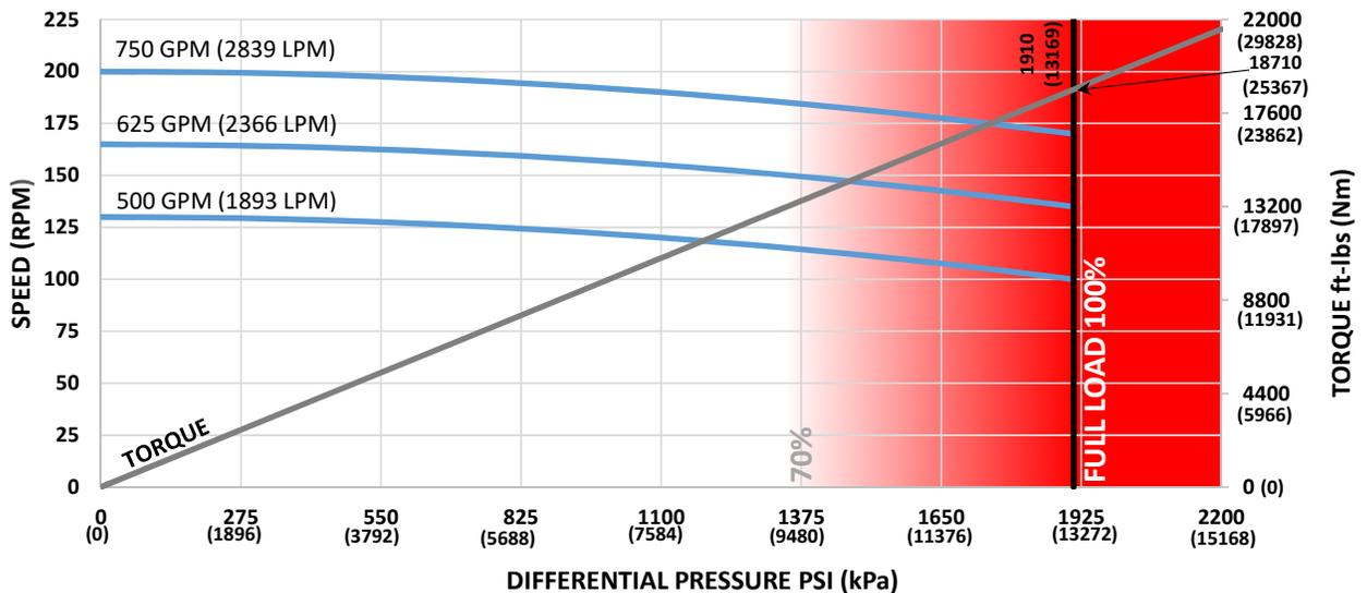
Possible damage may occur when motor is run higher than 70% of Maximum Differential Pressure.
