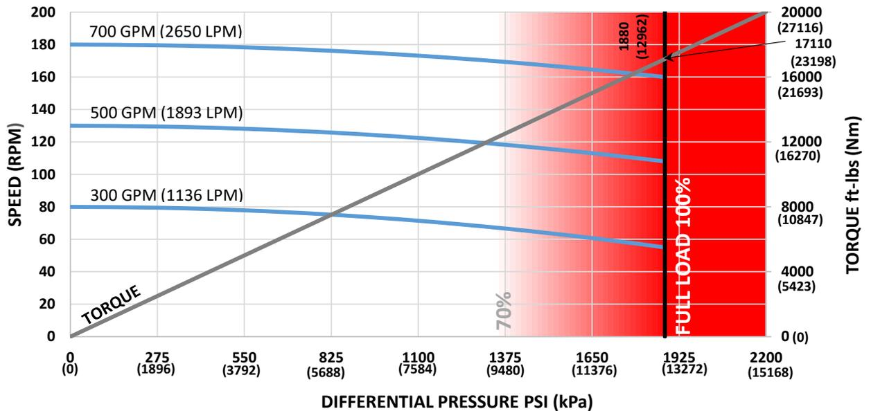
Possible damage may occur when motor is run higher than 70% of Maximum Differential Pressure.
